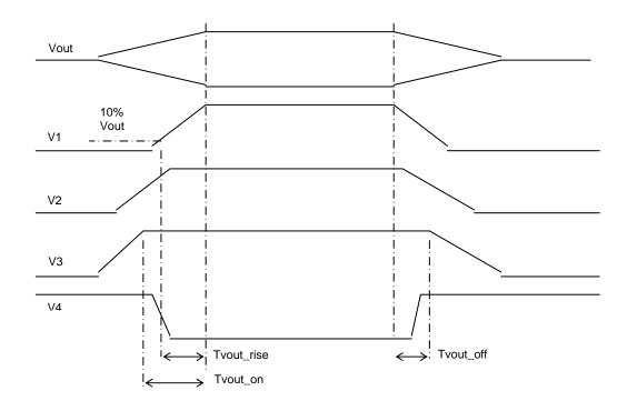
Figure 8. Output Voltage Timing
